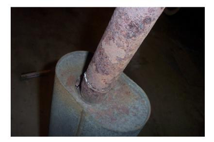
My first course of action was to remove all the loose rust. Using a wire brush I spent a good hour scraping all the rust off. There were sections of loose rust that needed to be chipped off as well. Most of the rust was on the piping and ends of the muffler. The muffler body was fairly rust free.
